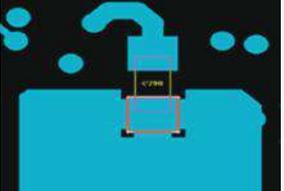
A close-up photograph of a component pad on a PCB. The pad is highlighted in blue, and the traces connecting it are highlighted in red. The traces have different widths.            | DIFFERENT TRACE WIDTHS CONNECTING PADS / SMALL PIN AREA - PAD AREA MAX- CAN CAUSE TOMBSTONING, KINDLY CHECK                               | OPEN   |                   |
