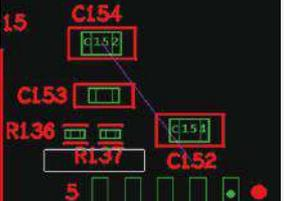
A top-down view of a PCB layout with several components highlighted in red. The reference designators are C154, C153, R136, R137, C152, and 5.                                      | COMPONENTS WITH MISPLACED REFERENCE DESIGNATORS ON THE SILKSCREEN CAN CAUSE ERRORS AT RE-WORK                                             | OPEN   |                   |
