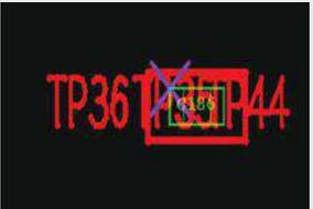
A photograph of a PCB silk screen with several areas highlighted in red. The text 'TP36' and 'P44' are visible, along with some illegible characters.                               | SILK SCREEN CLEAN UP IS NOT PROPER KINDLY CHECK.                                                                                          | OPEN   |                   |
